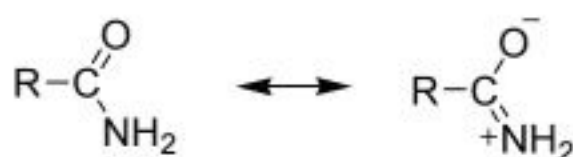
Figure 4.2 Resonance structures of amides
